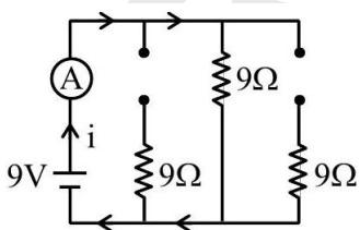
$\text{at } t = 0 \text{ all inductors act as open circuit } i = \frac{9}{9} = 1 \text{ A}$
